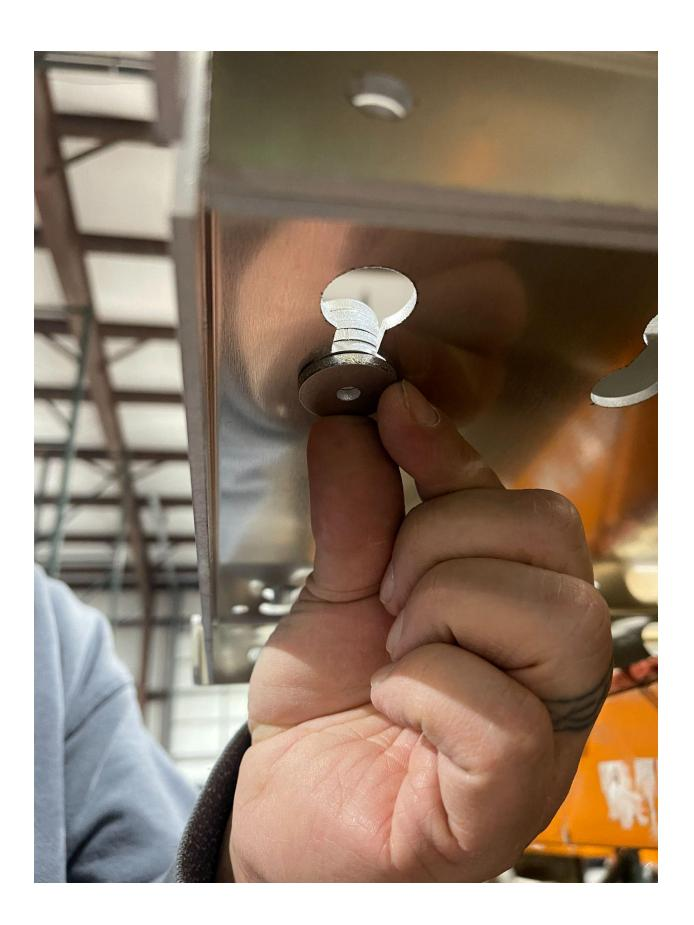
5. Then you'll use the M6x30 countersunk bolts to put through the top corner if it's a JK Cargo Shelf and the one below that if it's a JL Cargo Shelf. You'll then put the M6 Nyloc Nut on the bottom.
