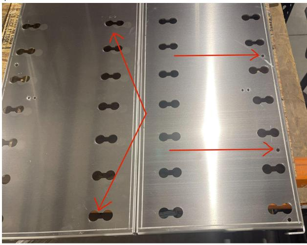
3. Using the M6x14 button head bolts and 2 M6 Nyloc Nuts you will install the front two bolts through the slanted portion of the Red box Mounting plate into the existing holes where the edge guard used to be.
